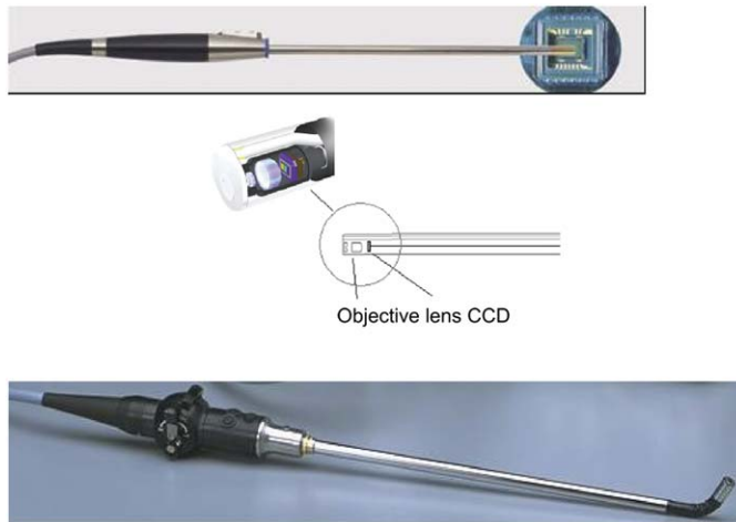
Fig. 2. Chip on a stick or EndoEye technology. This technological advance allowed for the development of the flexible laparoscope. (From Olympus America, Melville, New York.)
