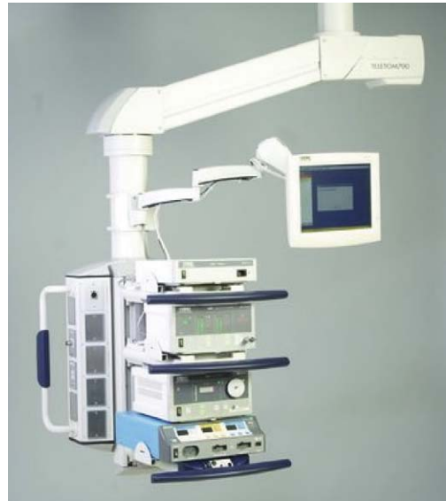
Fig. 7. Video carts (wheeled or suspended, as shown here) contain video camera electronics, light source, and various recording devices.
