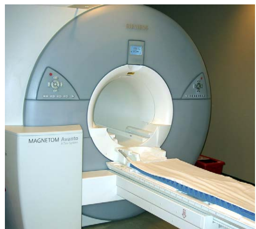
Fig. 1. MR scanner. The bore of the MRI scanner's magnet is the central opening where the strong magnetic field is generated.
